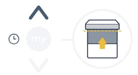
e. You can fine tune the position by briefly pressing the Up or Down buttons to ensure the upper limit is in the perfect position.
