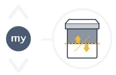
2. Press and hold the 'My' button on the remote until the motor moves the blind up and down.
