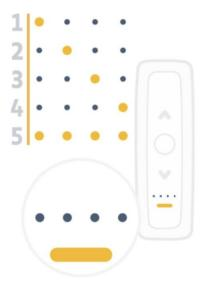
b. Ensuring you are on the correct channel, press the Up and Down buttons together until the motor shunts up and down.
