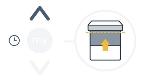
f. You can fine tune the position by briefly pressing the Up or Down buttons to ensure the upper limit is in the perfect position.
