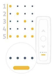
Briefly press the program button on the motor drive head, take notice of how many up and down movements occur. This will be either 0, 1, 2 or 3 jogs up and down.
