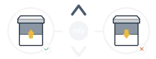
d. If the blind moves down, press and hold the 'My' button until the blind moves up and down. This will change the direction of the motor. Up will now be Up.
