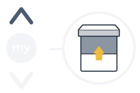
b. Press the Up and Down buttons together until the motor shunts up and down.
